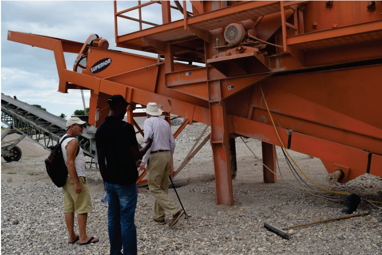
This is the upper end of the vibrating screen washer unit.
